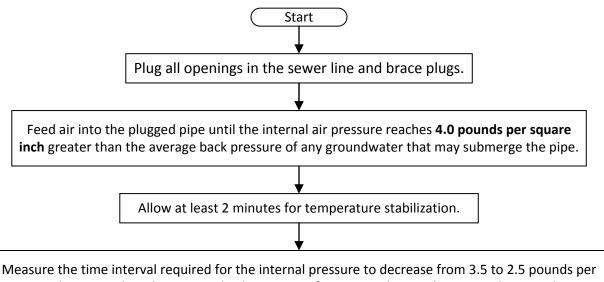
Testing Pass Criteria: Fulfill the minimum test time requirements as calculated by Ramseier's Equation below.
